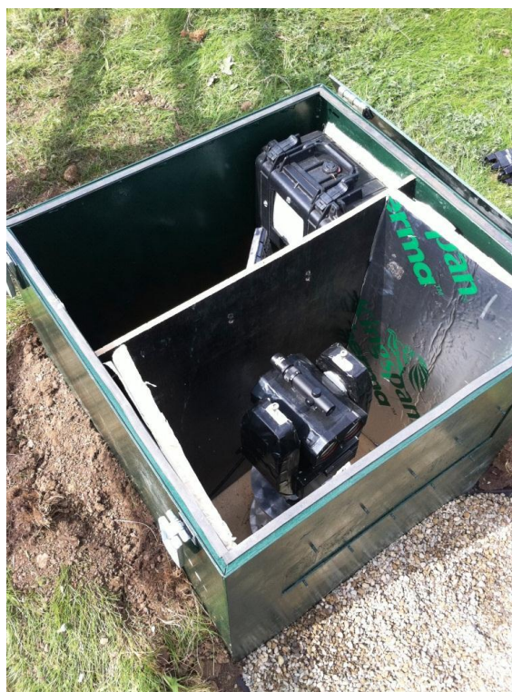
Figure 12 View inside the permanent scanner installation, showing the scanner nearest to the window mechanism, and the controls PC at the rear of the box
